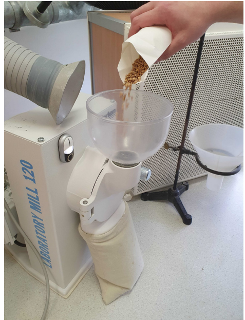
Figure 3. Wheat grain being milled to powder at Lantmännen's lab location to prepare for grain cadmium estimation. Photograph by Magda Karlo.
